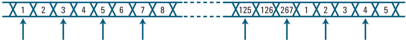
Figure 2. PRBS-7 with a length of 2^7-1 = 127 bits, under-sampled by 1:2; samples taken marked by arrows
